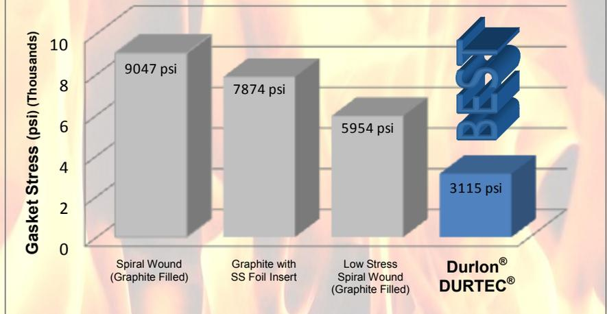
Values are based on an ANSI 4" Class 150 Ring Gasket with commonly published gasket factors. T3 (tight) represents a mass leak rate per unit diameter ( $L_{RM}$ ) of 0.00002 mg/sec-mm of gasket outside diameter. Durlon® is a registered trademarks of Gasket Resources, Inc.
