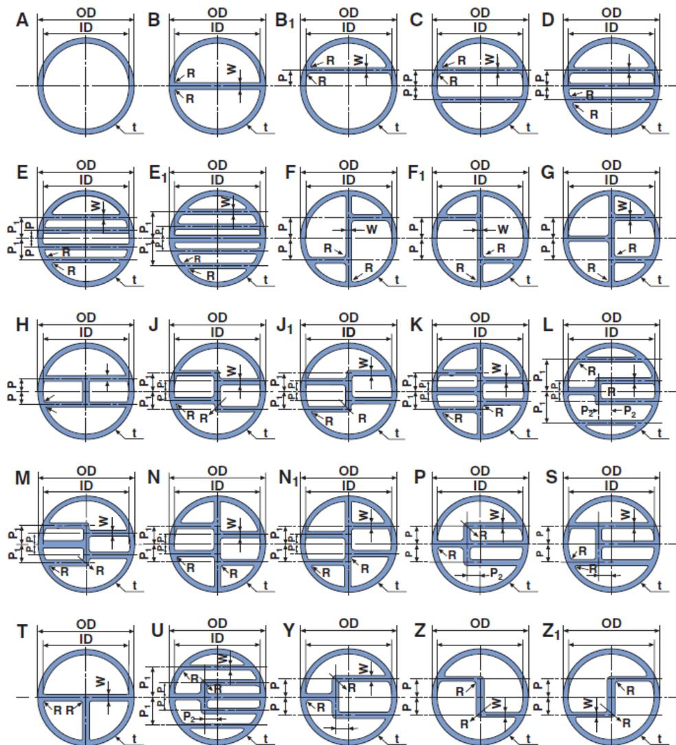
When inquiring and ordering, please specify the gasket shape by using the letter beside the style of the gasket as shown above. Along with the ID, OD, and thickness, we will require corner radii, flange width, distance from the center of the rib to the center of the gasket, and additional dimensions.
